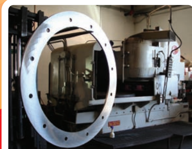
Blanchard - Our 60 inch chuck will cut stock quickly and allows us to grind parts up to 72" diagonally.
